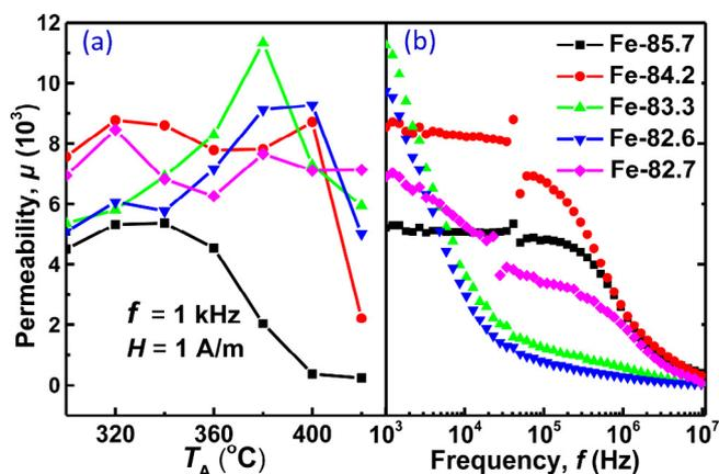
Fig. 2. (a) The dependence of effective permeability ( $\mu_e$ ) on  $T_A$  at a frequency ( $f$ ) of 1 kHz and 1 A/m for  $\text{Fe}_{(82.6-85.7)}\text{Si}_{(2-4.9)}\text{B}_{(9.2-11.2)}\text{P}_{(1.5-2.7)}\text{C}_{0.8}$  amorphous alloys. (b) The dependence of effective permeability ( $\mu_e$ ) on  $f$  of samples treated by longitudinal FA at 380 °C for 15 min.
