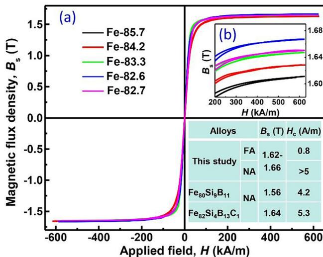
Fig. 4. (a) Hysteresis loops for  $\text{Fe}_{(82.6-85.7)}\text{Si}_{(2.4-9)}\text{B}_{(9.2-11.2)}\text{P}_{(1.5-2.7)}\text{C}_{0.8}$  amorphous alloys subjected to a longitudinal FA. (b) Inset of the partial amplified hysteresis loops. The insert table shows the  $B_s$  and  $H_c$  of the present alloys for a normal annealing (NA) and a magnetic field annealing (FA), as well as the commercial alloys.
