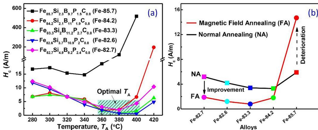
Fig. 1. (a) The dependence of  $H_c$  on  $T_A$  of  $\text{Fe}_{(82.6-85.7)}\text{Si}_{(2-4.9)}\text{B}_{(9.2-11.2)}\text{P}_{(1.5-2.7)}\text{C}_{0.8}$  amorphous alloys treated by longitudinal magnetic field annealing (FA) with an applied field of  $1.6 \times 10^3$  A/m and (b) the difference of  $H_c$  for FA and normal field-free annealing (NA) at the optimal  $T_A$ .
