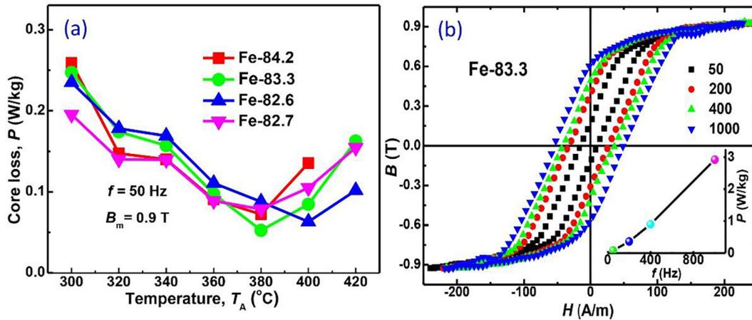
Fig. 3. (a) Core loss as a function of  $T_A$  for  $\text{Fe}_{(82.6-84.2)}\text{Si}_{(2.4-9)}\text{B}_{(9.2-11.2)}\text{P}_{(1.5-2.7)}\text{C}_{0.8}$  amorphous alloys treated by longitudinal FA, (b) the AC B-H hysteresis loops for the annealed  $\text{Fe}_{83.3}\text{Si}_{2}\text{B}_{11.2}\text{P}_{2.7}\text{C}_{0.8}$  alloy measured at different frequencies ( $f$ ).
