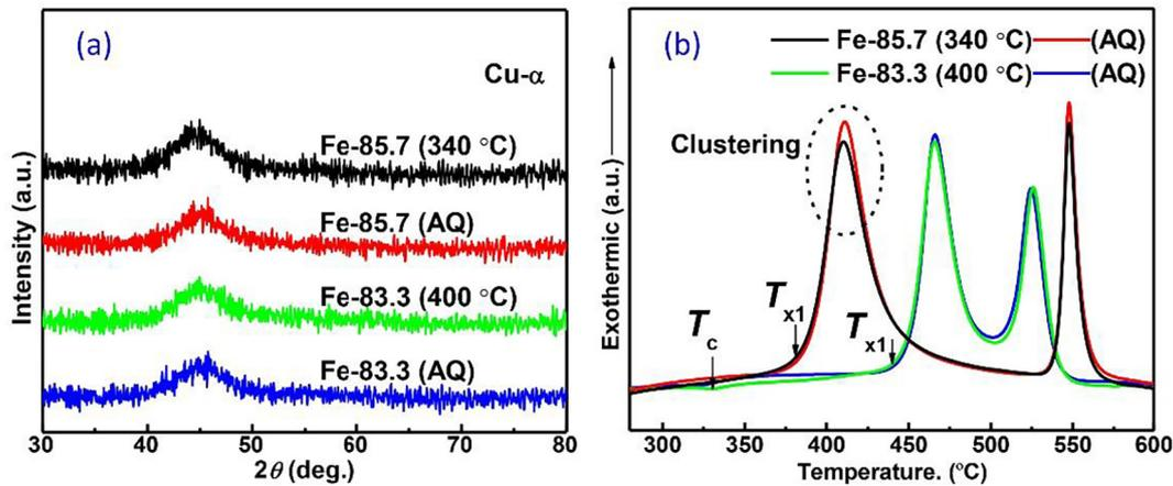
Fig. 6. (a) XRD patterns and (b) DSC curves of  $\text{Fe}_{83.3}\text{Si}_2\text{B}_{11.2}\text{P}_{2.7}\text{C}_{0.8}$  and  $\text{Fe}_{85.7}\text{Si}_{2.3}\text{B}_{9.7}\text{P}_{1.5}\text{C}_{0.8}$  alloy ribbons with different states.
