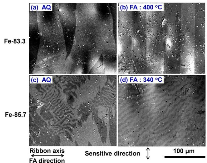
Fig. 5. Images of magnetic domain structures of  $\text{Fe}_{83.3}\text{Si}_{2}\text{B}_{11.2}\text{P}_{2.7}\text{C}_{0.8}$  and  $\text{Fe}_{85.7}\text{Si}_{2.3}\text{B}_{9.7}\text{P}_{1.5}\text{C}_{0.8}$  alloy ribbons with different states.
