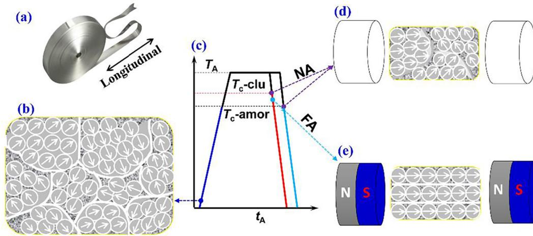
**Fig. 7.** (a) Applied field direction along the ribbon axial; (b) A sketch of magnetic domain structures of as-quenched ribbon; (c) Magnetic state of the amorphous alloys and clusters in the annealing process; (d) and (e) are the variation of magnetic moment and domain structure for the annealed ribbon by a normal field-free annealing (NA) and a longitudinal magnetic field annealing (FA), respectively.
