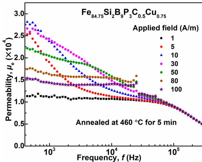
Fig. 7. The changes of  $\mu_e$  as a function of frequency at different  $H_m$  from 400 Hz to 200 kHz for the  $\text{Fe}_{84.75}\text{Si}_2\text{B}_9\text{P}_3\text{C}_{0.5}\text{Cu}_{0.75}$  nanocrystalline alloy.
