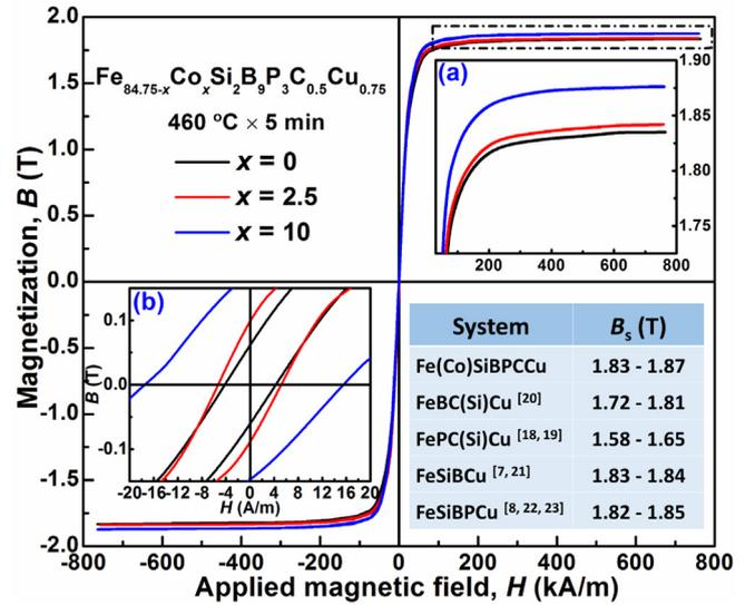
Fig. 5. Hysteresis loops of the  $\text{Fe}_{84.75-x}\text{Co}_x\text{Si}_2\text{B}_9\text{P}_3\text{C}_{0.5}\text{Cu}_{0.75}$  ( $x = 0, 2.5$  and  $10$ ) ribbons after annealing at optimum conditions; Inset (a) partially enlarged hysteresis loops; Inset (b) partially enlarged  $B$ - $H$  loops; Inserted table shows the  $B_s$  for the typical nanocrystalline alloy systems.
