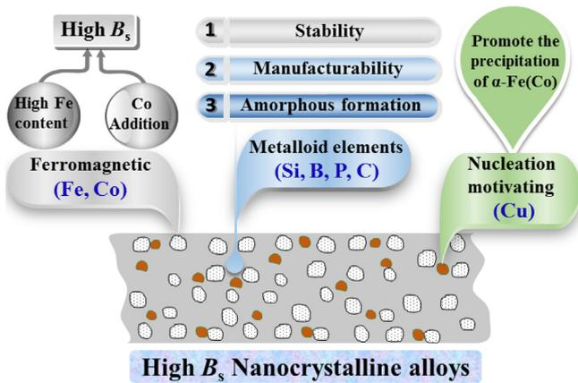
Fig. 1. The composition design of the  $\text{Fe}_{84.75-x}\text{Co}_x\text{Si}_2\text{B}_9\text{P}_3\text{C}_{0.5}\text{Cu}_{0.75}$  high  $B_s$  nanocrystalline alloys.
