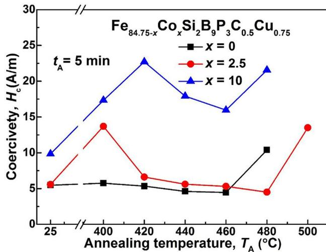
Fig. 4.  $H_c$  of the  $\text{Fe}_{84.75-x}\text{Co}_x\text{Si}_2\text{B}_9\text{P}_3\text{C}_{0.5}\text{Cu}_{0.75}$  ( $x = 0, 2.5$  and  $10$ ) ribbons dependence on  $T_A$  after annealing for 5 min.
