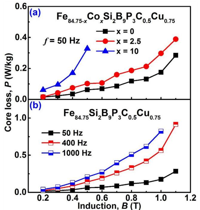
Fig. 6. Core loss of the ribbons after annealing at  $460^\circ\text{C}$  for 5 min; (a)  $\text{Fe}_{84.75-x}\text{Co}_x\text{Si}_2\text{B}_9\text{P}_3\text{C}_{0.5}\text{Cu}_{0.75}$  ( $x = 0, 2.5$  and  $10$ ) alloy ribbons were measured at 50 Hz; (b)  $\text{Fe}_{84.75}\text{Si}_2\text{B}_9\text{P}_3\text{C}_{0.5}\text{Cu}_{0.75}$  alloy ribbons were measured at 50 Hz, 400 Hz and 1000 Hz, respectively.
