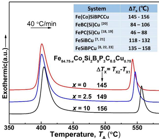
Fig. 3. DSC traces of the as-quenched  $\text{Fe}_{84.75-x}\text{Co}_x\text{Si}_2\text{B}_9\text{P}_3\text{C}_{0.5}\text{Cu}_{0.75}$  ( $x = 0, 2.5$  and  $10$ ) ribbons; Inserted table shows the  $\Delta T_x$  of the typical nanocrystalline alloy systems.
