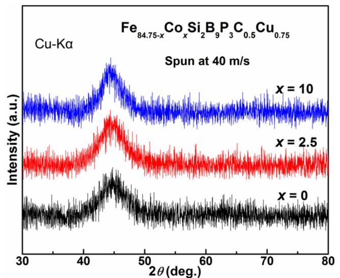
Fig. 2. XRD patterns of the as-quenched  $\text{Fe}_{84.75-x}\text{Co}_x\text{Si}_2\text{B}_9\text{P}_3\text{C}_{0.5}\text{Cu}_{0.75}$  ( $x = 0, 2.5$  and  $10$ ) ribbons.
