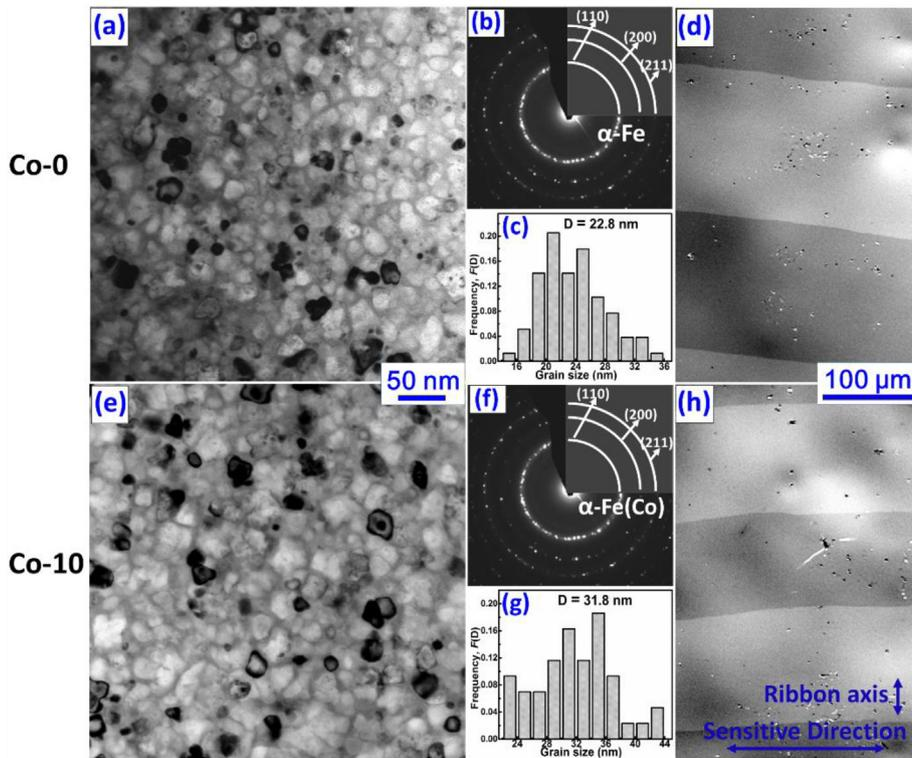
**Fig. 9.** TEM bright field images, SAED patterns and grain size distribution for the  $\text{Fe}_{84.75-x}\text{Co}_x\text{Si}_2\text{B}_9\text{P}_3\text{C}_{0.5}\text{Cu}_{0.75}$  alloy (a–c)  $x = 0$  and (e–g)  $x = 10$ ; Magnetic domains of (d)  $x = 0$  and (h)  $x = 10$  ribbons after annealing under optimal temperature, respectively.
