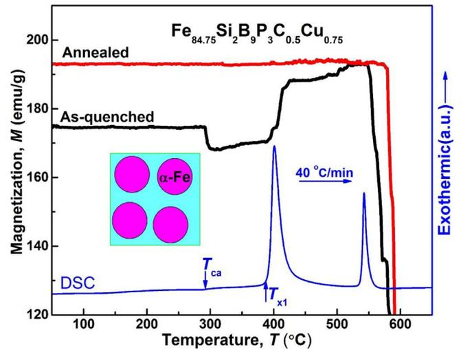
Fig. 8. Magnetization as a function of temperature for the  $\text{Fe}_{84.75}\text{Si}_2\text{B}_9\text{P}_3\text{C}_{0.5}\text{Cu}_{0.75}$  ribbons after annealing under optimum conditions and as-quenched ribbons.
